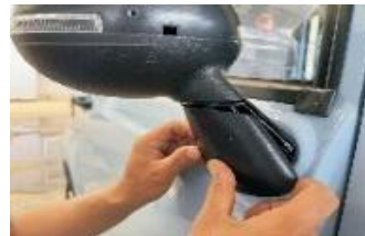
Fig. 10 • Securing and finishing the mirror assembly.
