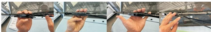
Fig. 11 · Connecting the wiper blade and washer hose.
