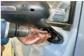
Fig. 10 • Securing and finishing the mirror assembly.
