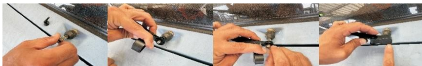
Fig. 12 · Fitting to the wiper mounting.
