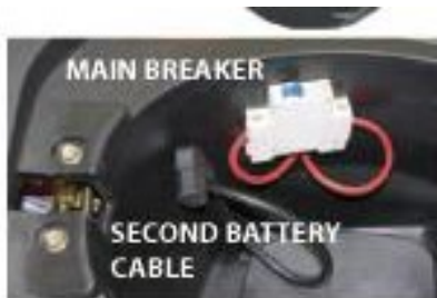
Fig. 7 · Main switch in the area below the seat.
