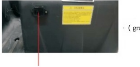
Charging inlet on the right-hand side.
